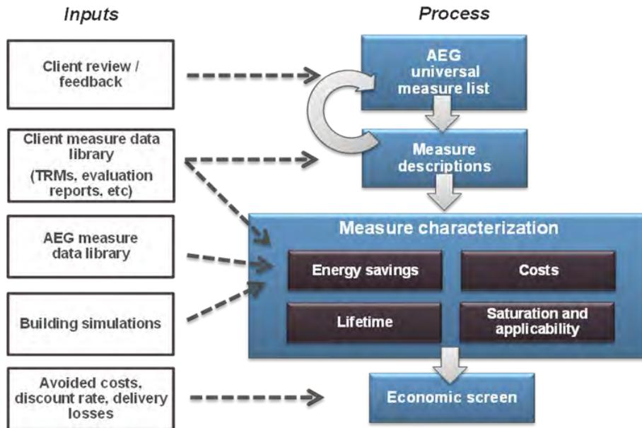
Figure 1-1 Approach for Energy Efficiency Measure Assessment
