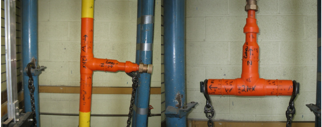
Photograph #11 Pull testing T-main segments (Photograph taken by Staff)
