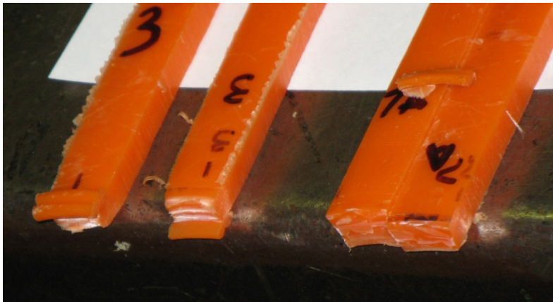
Photograph #12 Segment 1N failure inside fusion area (Photograph taken by Staff)
