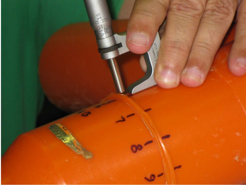
Photograph # 6—Fusion bead height measurement testing (Photograph taken by Staff)
