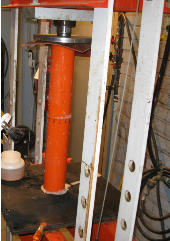
Photograph #7—Pressure test with air medium (Photograph taken by Staff)
