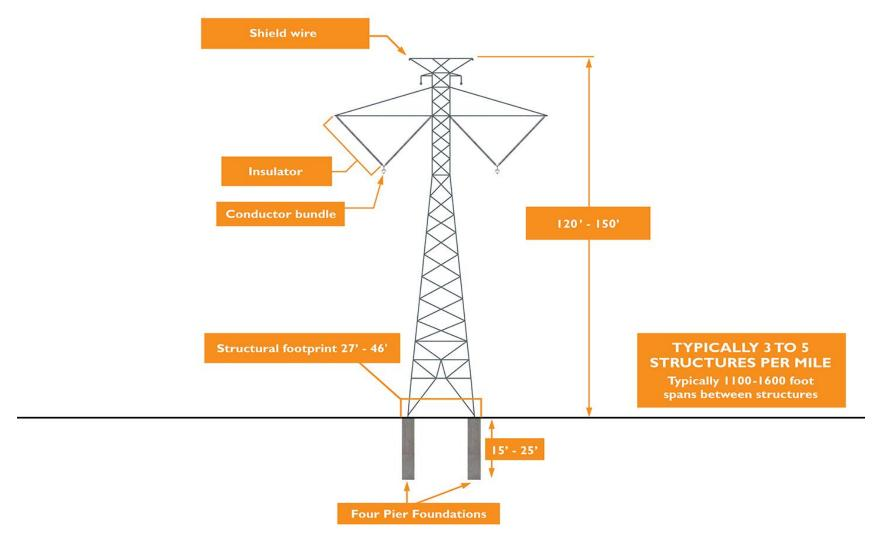
Schedule JLA-4c. Average specifications for a typical steel lattice transmission structure. The average foundation footprint for a typical steel lattice transmission structure is 28 feet on a side and is roughly square, resulting in a direct conversion of approximately 784 square feet or .018 acres of cropland per structure.
