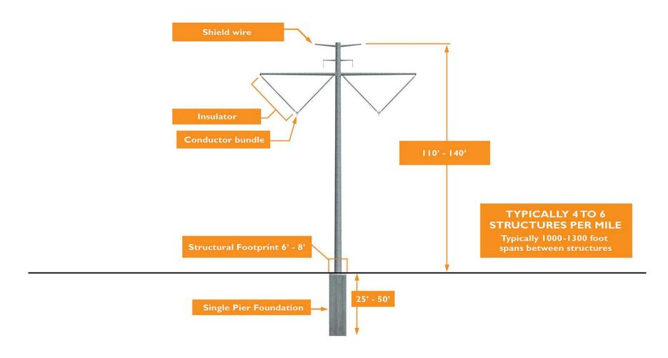
Schedule JLA-4a. Average specifications for a typical steel monopole structure. The average foundation footprint for a typical steel monopole transmission structure is 7 feet in diameter and is roughly circular, resulting in a direct conversion of approximately 39 square feet or .0009 acres of cropland per structure.
