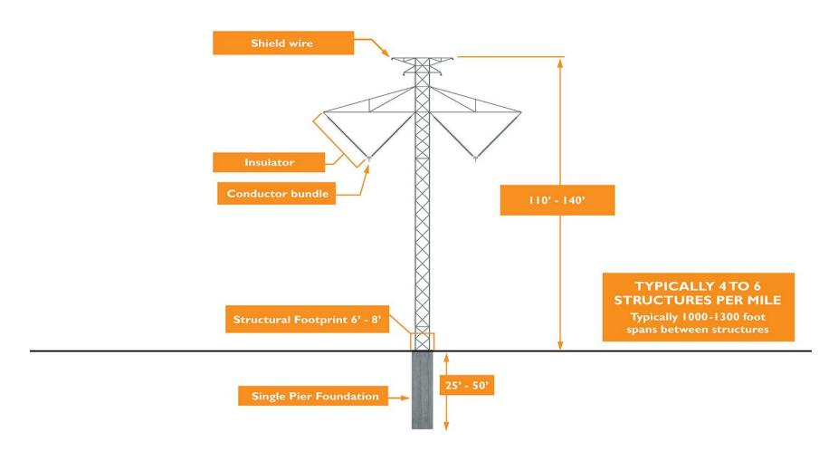
Schedule JLA-4b. Average specifications for a typical steel lattice mast structure. The average foundation footprint for a typical steel monopole transmission structure is 7 feet in diameter and is roughly circular, resulting in a direct conversion of approximately 39 square feet or .0009 acres of cropland per structure.
