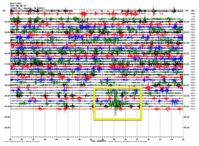
The M4.0 Poplar Bluff earthquake on November 17, 2021 was recorded at an earthquake monitoring station at the CUSEC headquarters in Memphis, Tennessee. The station, along with many others in the region, is operated and monitored by the <u>Center for Earthquake Research</u> and Information (CERI) at the University of Memphis.
