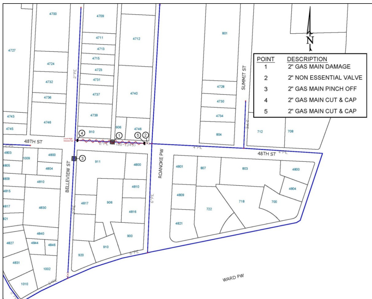
Figure 5 – Actions Taken to Isolate the Damaged Section of Main on W. 48 th Street (Provided by MGE)
