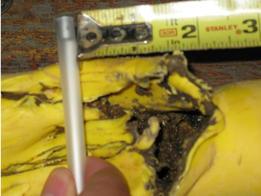
Photograph #1 – Approximate 2-inch wide hole in damaged section of main oriented west (left side) to east (right side) (Staff Photo)
