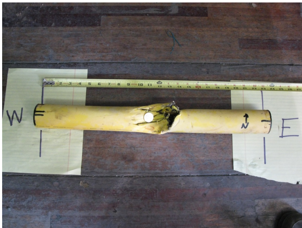
Photograph #22 – Section of damaged main that was removed. A quarter was placed on the removed section of main as a reference to the size of the damage. (Staff Photo)
