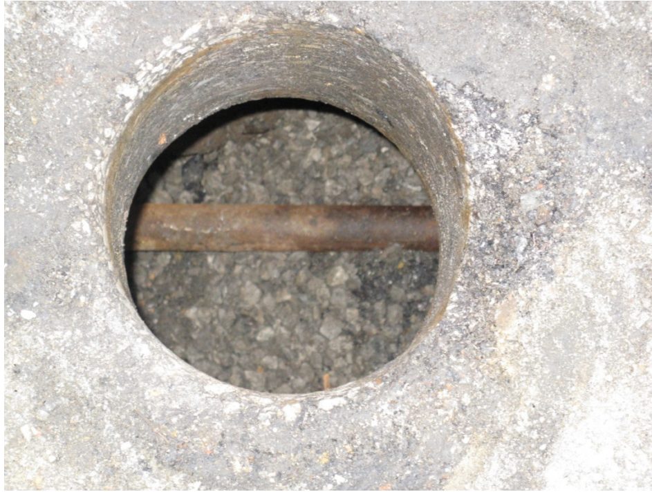
Photograph #17 – Boring rod seen in one of potholes located near the northeast corner of JJ's Restaurant (Staff Photo).
