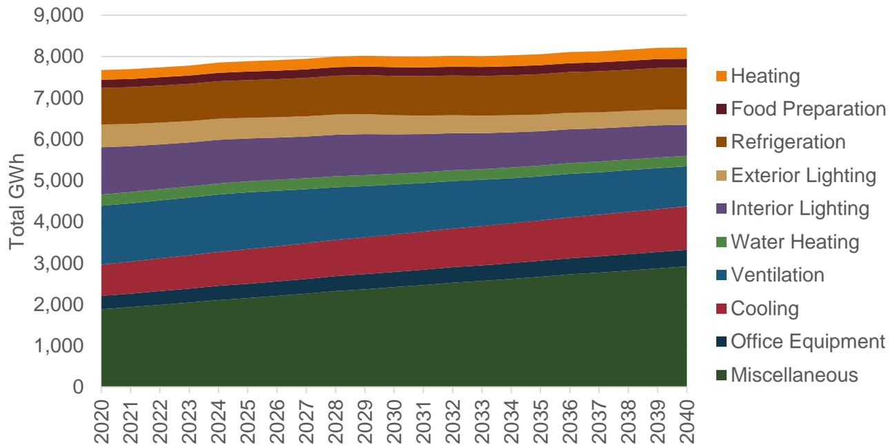
Figure I-15 Evergy commercial baseline electricity projection by end use
