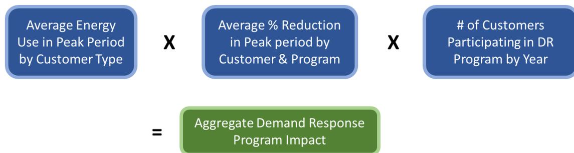
Figure II-1 DR/DSR potential evaluation—basic principle
