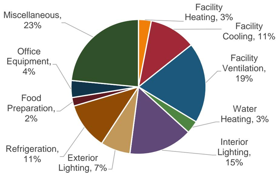
Figure I-5 Evergy commercial electricity use by end use, 2019
