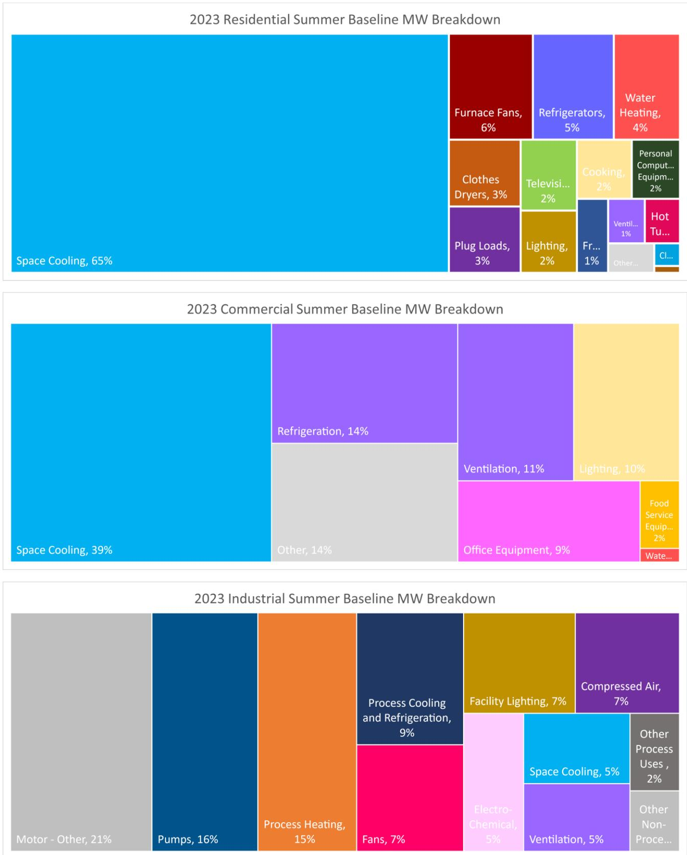
Figure II-7 Sector-wise end-use level breakdown of peak summer load
