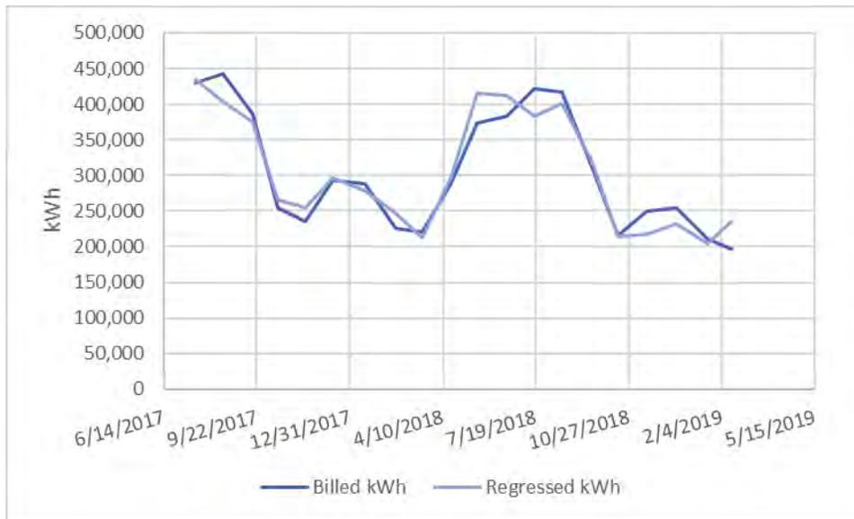
Annual kWh savings for the installed measures were determined by using typical year (TMY3) weather data and the derived equation to calculate monthly pre/post energy consumption of the site. Each month was summed for a year to obtain annual energy savings. Annual kWh savings are the difference between baseline and as-built energy consumption for the facility, and can be seen in the following table:
