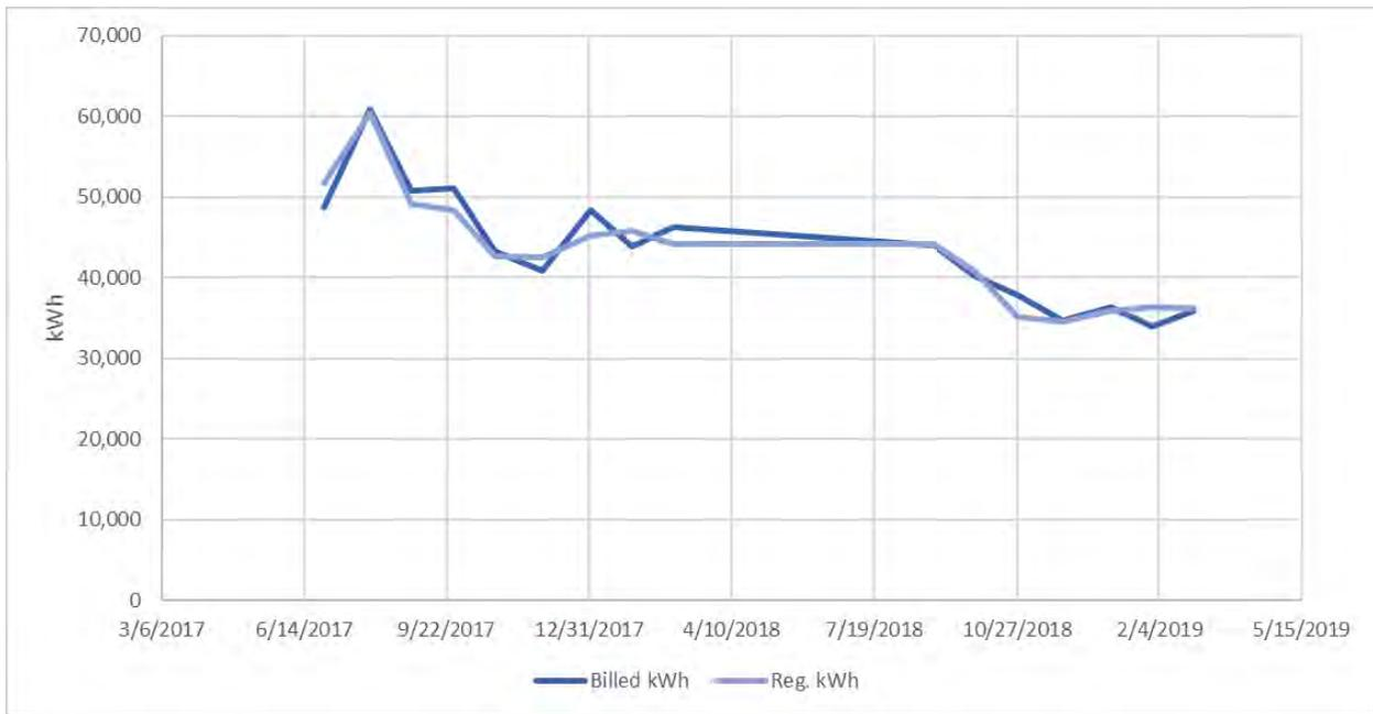
Annual kWh savings for the installed measures were determined by using typical year (TMY3) weather data and the derived equation to calculate monthly pre/post energy consumption of the site. Each month was summed for a year to obtain annual energy savings. Annual kWh savings are the difference between baseline and as-built energy consumption for the facility, and can be seen in the following table:
