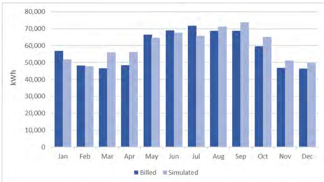
Upon the calibration of the as-built model using billing data, an alternative model run was utilized in Trane Trace to determine the energy impacts of the HVAC measures above ASHRAE 90.1-2007 Appendix G. The two models were run using typical weather (TMY3) for the region to determine the typical annual savings for the project. The annual savings are the difference between the annual
