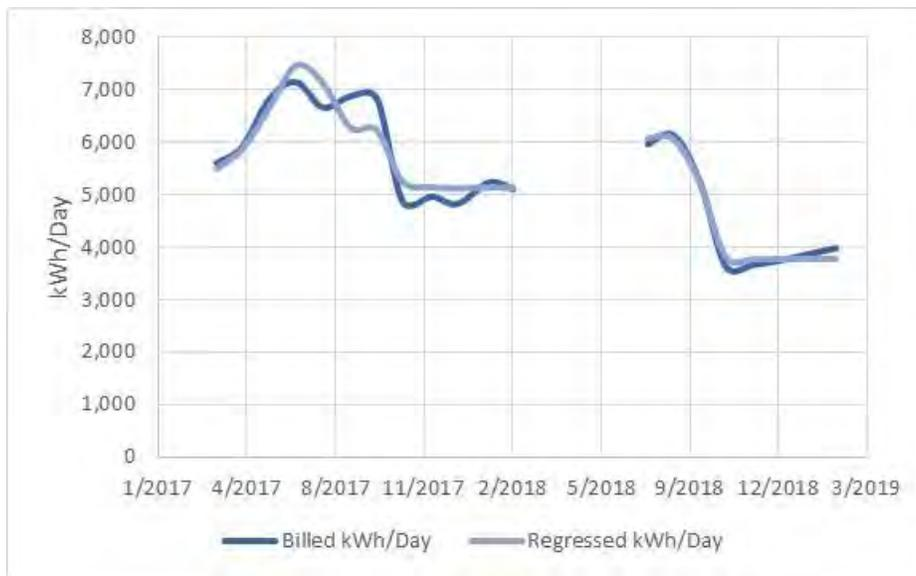
Annual kWh savings for the installed measures were determined by using typical year (TMY3) weather data and the derived equation to calculate monthly pre/post energy consumption of the site. Each month was summed for a year to obtain annual energy savings. Annual kWh savings are the difference between baseline and as-built energy consumption for the facility, and can be seen in the following table:
