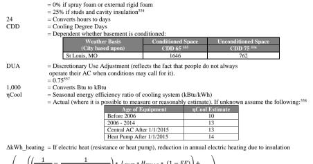
$$= \frac{\left(\left(\left(\frac{1}{R_{OldAG}} - \frac{1}{(R_{Added} + R_{OldAG})}\right)^* L_{BWT} * H_{BWAG} * (1 - FF)\right) + \left(\left(\left(\frac{1}{R_{OldBG}} - \frac{1}{(R_{Added} + R_{OldBG})}\right)^* L_{BWT} * (H_{BWT} - H_{BWAG}) * (1 - FF)\right)\right)}{* HDD * 24 * DUA * ADJ_{Basement}}$$
