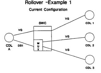
The customer requests that the voiceband circuit (VG) between CDL A and CDL 1 be "rolled over" to the DS1 serving CDL A. No NRCs apply for this request.
