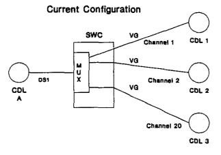
The customer requests that the voiceband circuit serving CDL 3 be moved from channel 20 in the DS1 serving CDL A to Channel 3 in the same DS1. No NRCs apply for this request.
