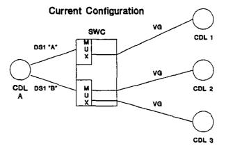
The customer requests that the voiceband (VG) circuit serving CDL 1 be moved from the DS1 "A" circuit to the DS1 "B" circuit. No NRCs apply for this request.
