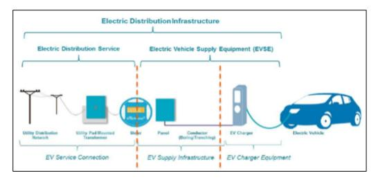
In general, EV infrastructure costs can be broken into three groups: the "EV Service Connection"; the "EV Supply Infrastructure"; and the "EV Charger Equipment." The EV Service Connection refers to that common utility distribution infrastructure, including transformers, utility services, and meters, which is ordinarily part of the regulated asset base. The EV Supply
