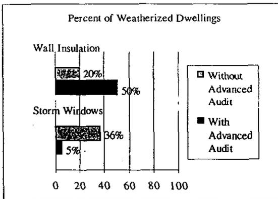
**Insulation** was the next most common type of energy conservation measure installed. Attic insulation was either used for the first time or added to existing insulation in the majority of homes receiving insulation. Wall insulation was installed in less than 20 percent of homes. Today, with the use of advanced audits, attic and, especially, wall insulation are installed much more frequently.
