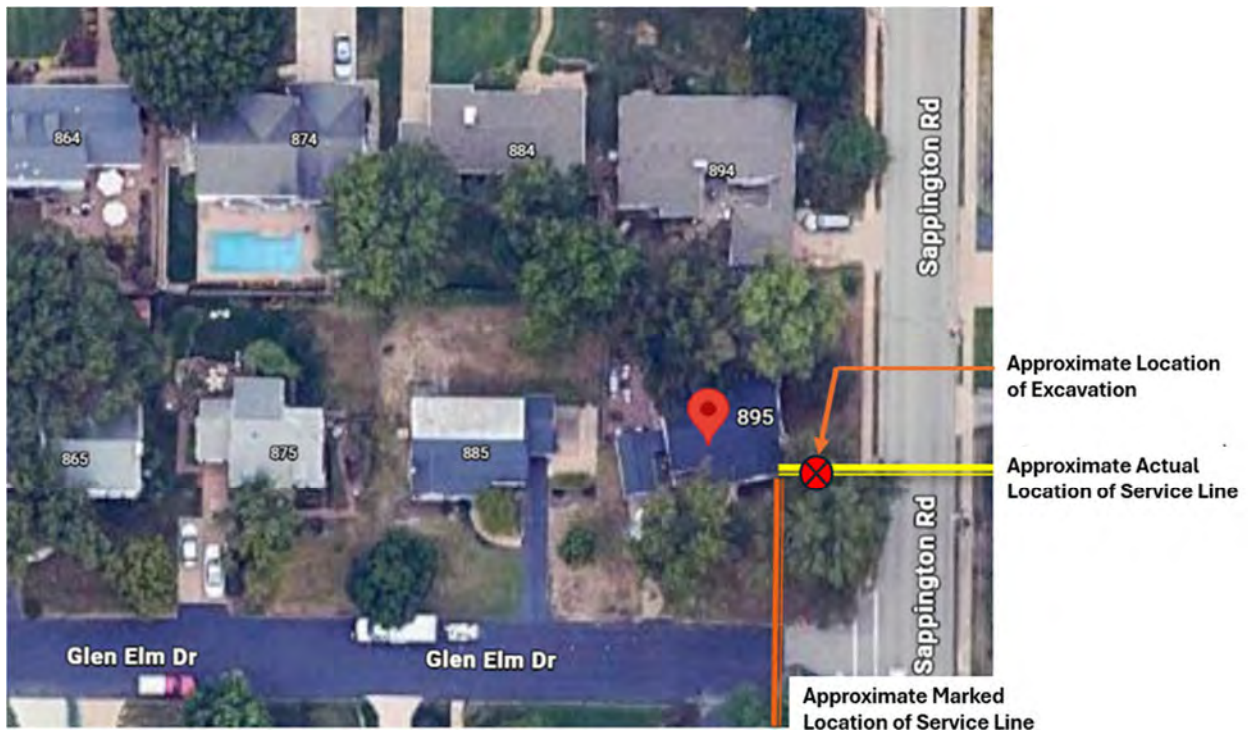
Figure 2: Approximate Locations of Actual Gas Service Line to 895 Glen Elm Dr., Excavation Location and Marked Location of Service Line on January 3, 2025 (Source: Google Maps, Staff added approximate locations of service line and text boxes).
