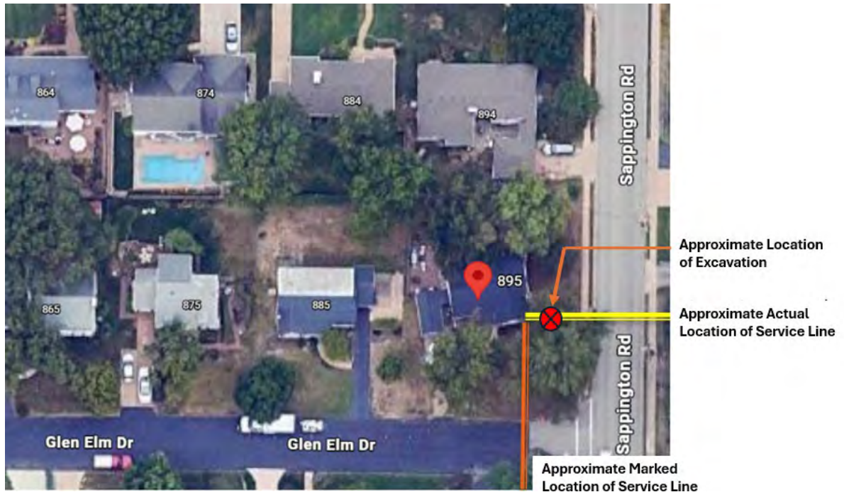
Figure 1: Approximate Locations of Actual Gas Service Line to 895 Glen Elm Dr., Excavation Location and Marked Location of Service Line on January 3, 2025 (Source: Google Maps, Staff added approximate locations of service line and text boxes).
