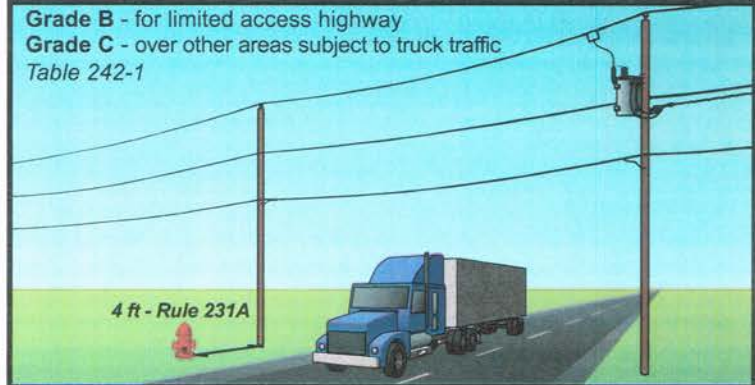
Vertical Clearance at Largest Vertical Sag Table 232-1
