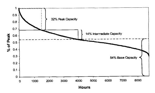
The utility in the graph above has a higher load factor than the utility shown below. It shows that this utility should have approximately 54% of its generation capacity base load, 14% intermediate and 32% peak.
