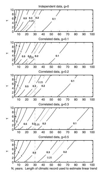
FIG. 4. Estimates of  $\eta(N, g, \tau)$ , the error for extrapolated expected value  $Y(t_0 + \tau)$  beyond the end of time interval of N yr utilized to estimate parameters of linear trend;  $\tau$  is in years.
