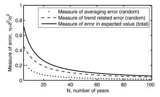
FIG. 3. Estimates of  $\eta(N, g = 0.2, \tau = 0)$ , the error in expected value  $Y(t_0)$  at the end of time interval N yr utilized to estimate parameters of linear trend (black line). Dotted and dashed lines show separately the averaging and the trend-related components of error variance.
