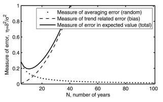
FIG. 2. Optimal climate normals:  $\eta(N, g = 0.2, \beta = 0.05, \tau = 0)$ —the error of expected value  $Y(\tau = 0)$  at the very end of an averaging time interval of N yr for a specified linear trend  $\beta = 0.05$  and lag-1 autocorrelation g = 0.2 (solid line). Dotted and dashed lines show separately the averaging  $\eta_a(N, g = 0.2)$  and the trend-related  $\eta_b(N, \beta = 0.05, \tau = 0)$  components of the error.
