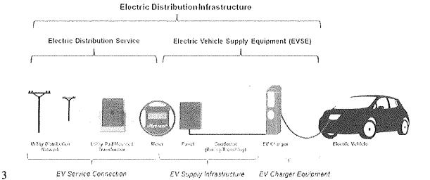
PEV infrastructure costs consist of three groups: the "EV Service Connection"; the "EV Supply Infrastructure"; and the "EV Charger Equipment." The EV Service Connection refers to the utility distribution infrastructure, including transformers, utility services, and meters. The EV Supply Infrastructure is comprised of the electricity panels, conduit and wiring.
