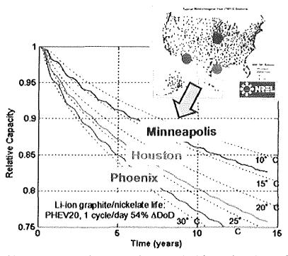
FIGURE 2-3 Effect of ambient temperature on battery capacity on a 20 kWh battery in a PHEV. NOTE: DoD, depth of discharge; PHEV, plug-in hybrid electric vehicle. SOURCE: Pesaran et al. (2013).
