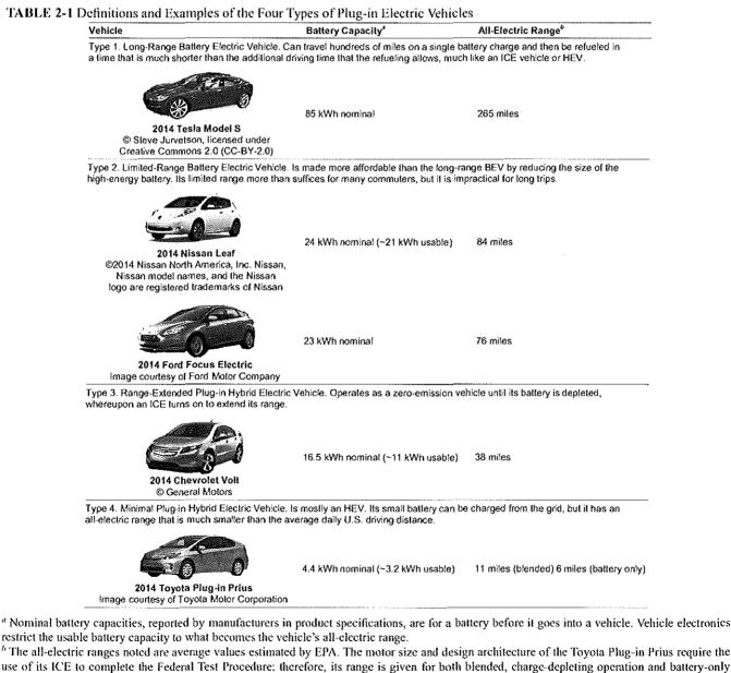
use of its ICE to complete the Federal Test Procedure: therefore, its range is given for both blended, charge-depleting operation and battery-only operation. All other vehicle ranges are given only for fully electric, charge-depleting operation. NOTE: HEV, hybrid electric vehicle; ICE, internal-combustion engine.
