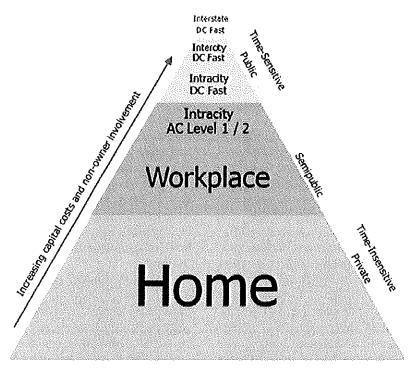
FIGURE 5-1 PEV charging infrastructure categories, ranked by their likely importance to PEV deployment, with the most important, home charging, on the bottom, and the least important, interstate DC fast charging, at the top. NOTE: AC, alternating current; DC, direct current.
