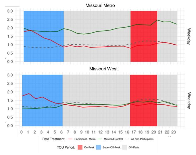
Figure 32. Winter EV Pilot Period Pilot Period Load Profiles
