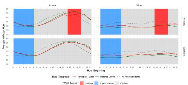
Figure A-40. eco+ Smart Thermostats Post-Period Load Shapes – Missouri West
